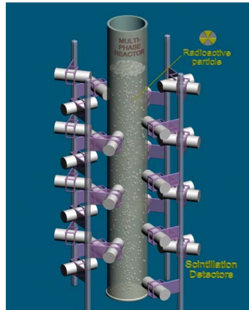
Figure 2. Diagram of CARPT Setup
