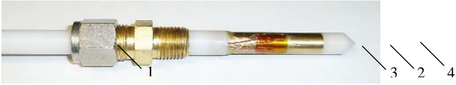
Figure 1. Picture of the heat transfer measurement probe 1: Teflon tube, 2: brass shell, 3: heat flux sensor, 4: Teflon cap.
