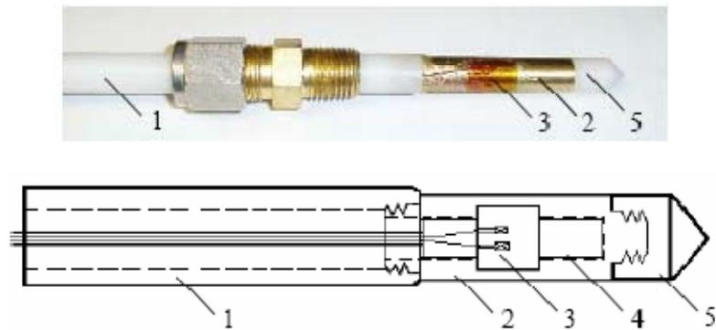
Figure 3-4. Photo and schematic diagram of the heat transfer probe
