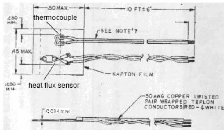
Figure 3-5. Schematic diagram of the heat flux sensor
