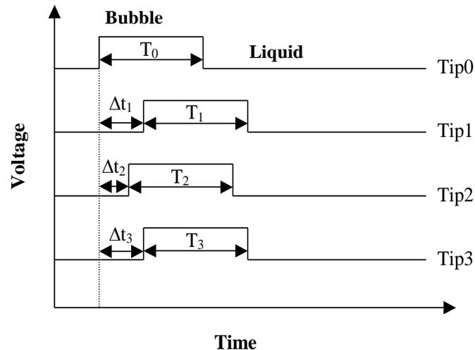
**Figure 3. Sketch of the Probe's Response to a Bubble Passing by**
