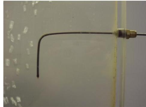
**Figure 2. The Four-point Optical Probe Installed in a 2D Bubble Column**
