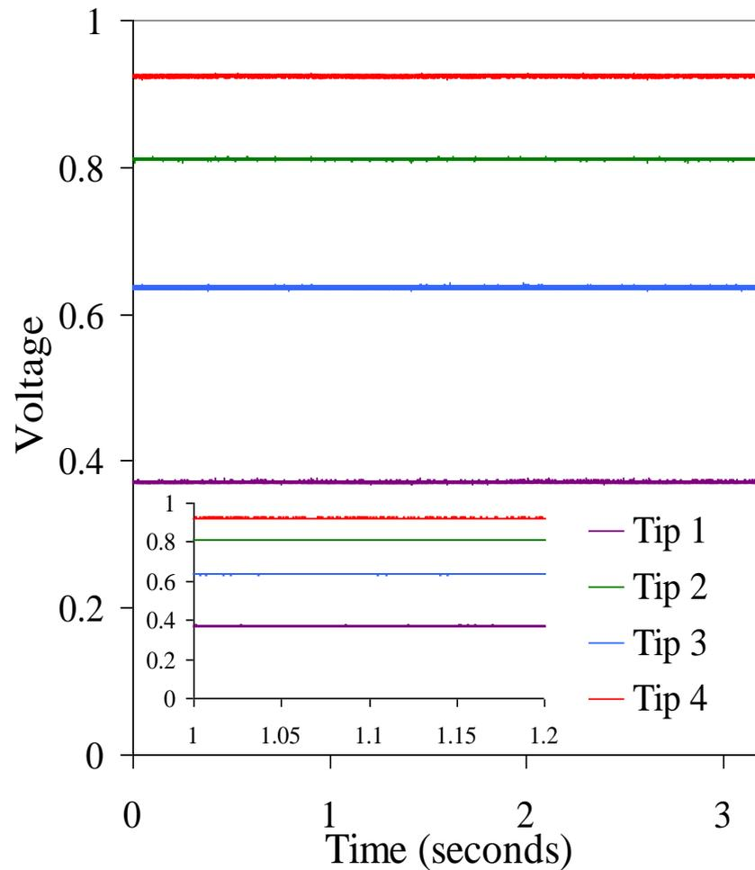
**Figure 7. Probe response for decane/CO<sub>2</sub> at 32 °C and ~1050 psi**
