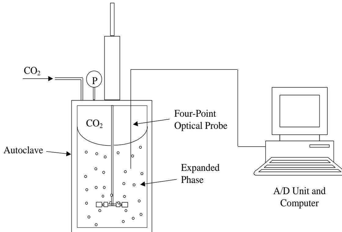
**Figure 5. Flow diagram of the application of the four-point optical probe in an autoclave stirred tank reactor for an expanded solvent/ $\text{CO}_2$  system.**
