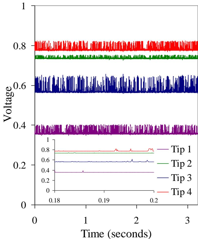
**Figure 6. Probe response for decane/CO<sub>2</sub> at 43 °C and ~1000 psi**
