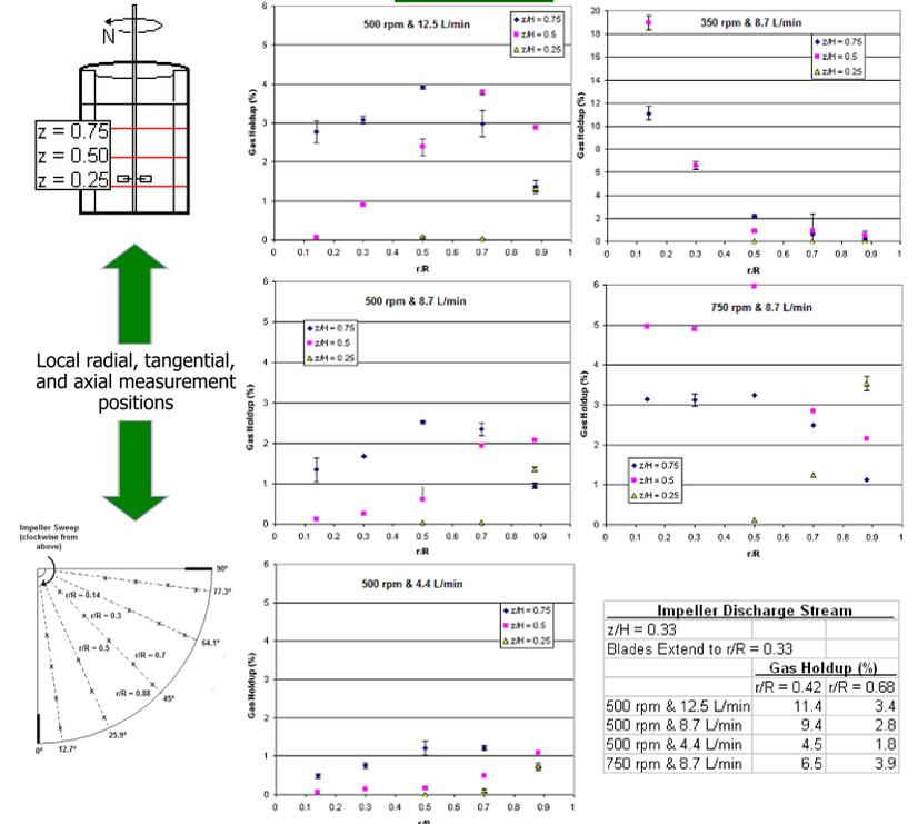
Optical probe accurately captures the complex 3D flow pattern in a multiphase stirred tank (local gas holdup, bubble size, bubble velocity vector, and specific interfacial area) and how it changes with operating conditions.
