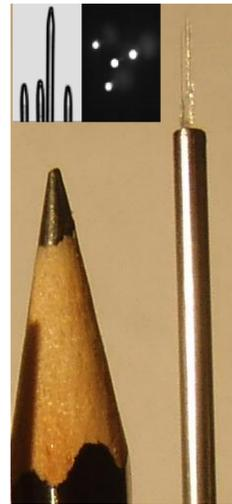
Improved working pressure and temperature of probe to 180 bar and 375 °C and reduced size to 0.625 mm for characterization of smaller bubbles
