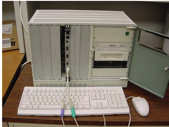
Figure B.23 PCI crate and single board computer.
