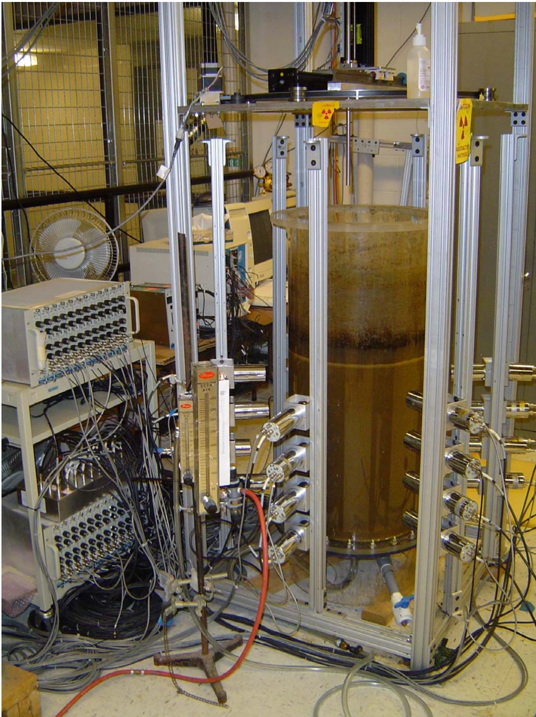
Figure 4.4 Photograph of CARPT set-up for pilot-scale digester
