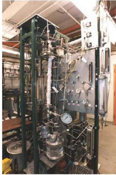
High pressure/high temperature packed bed facility
