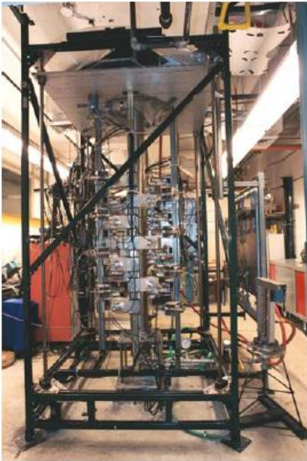
Computer automated radioactive particle tracking (CARPT)
