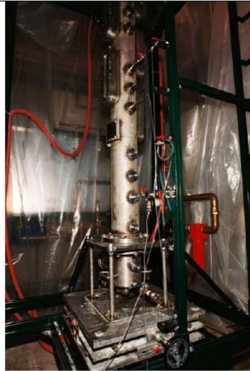
6-inch high pressure slurry bubble column with ports and windows
