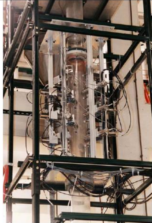
New CARPT facility mounted on gas-solid riser
