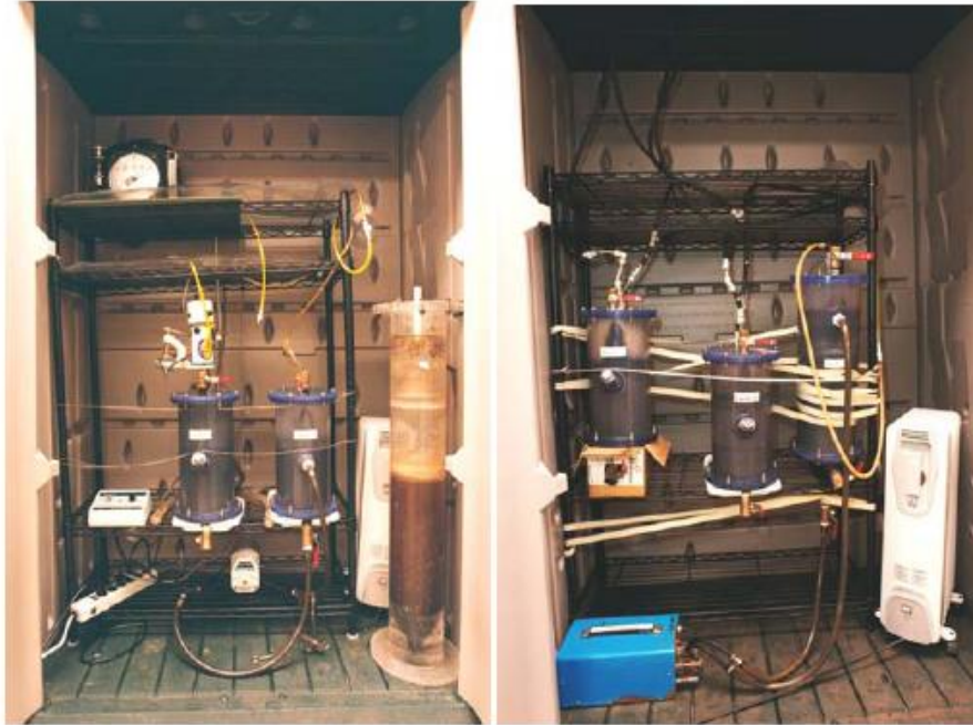
Anaerobic digesters inside temperature controlled cabinet
