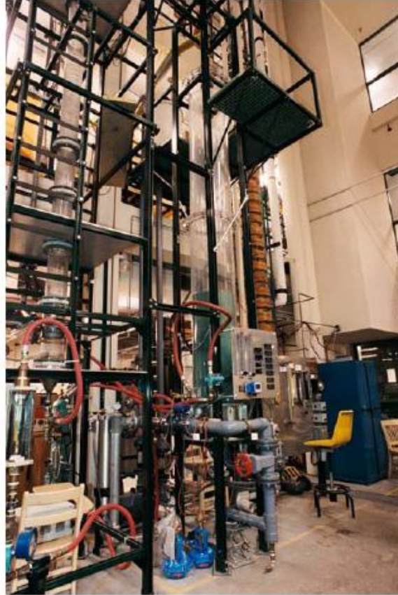
18-inch pilot plant scale ebullated bed, bubble and slurry bubble column
