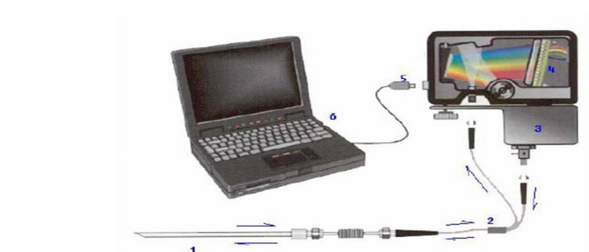
Optical oxygen probe system (Ocean Optics, Inc.) 1. Optical oxygen probe, 2. Optical fiber, 3. Light source, 4. Spectrometer, 5. Integrated A/D converter and USB interface, 6. PC and software
