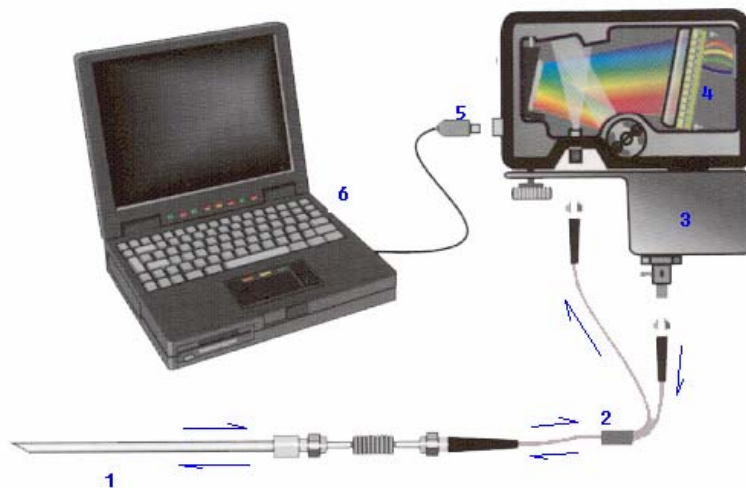
Figure 5-2. Optical oxygen probe system (Ocean Optics, Inc.) 1. Optical oxygen probe; 2. Optical fiber; 3. Light source; 4. Spectrometer; 5. Integrated A/D converter and USB interface; 6. PC and software
