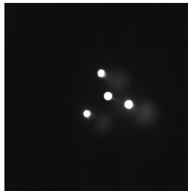
(b) Microphotograph showing bottom view of the four-point probe (not to scale, field of view 2 \times 2 mm)
